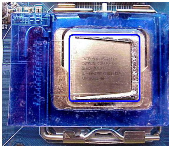
ETI on CPU lid with correct alignment and placement
